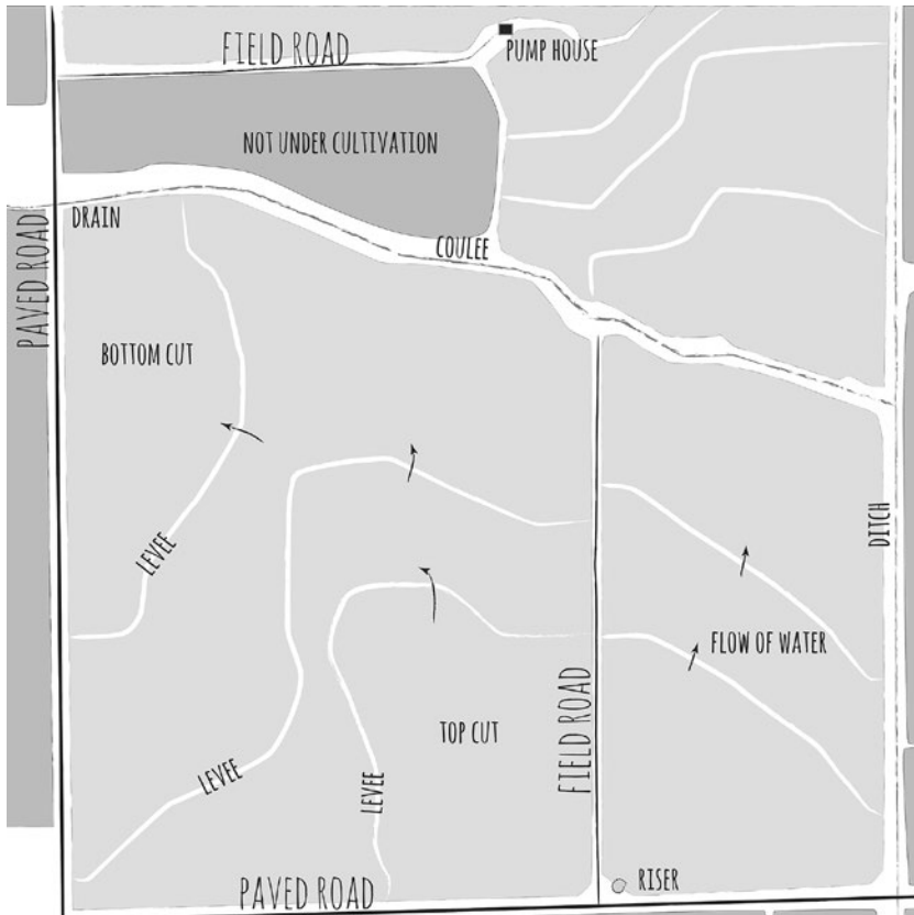
1.1. A plan of a rice field divided into cuts. Water is pumped into the top cut, or cuts, and then flows through the terraced levels via a series of gates, drains, or curtains to the bottom cut from which it drains into adjacent ditches, coulees, or bayous. While fields usually follow mapped survey boundaries, cut boundaries follow the land's topography.
