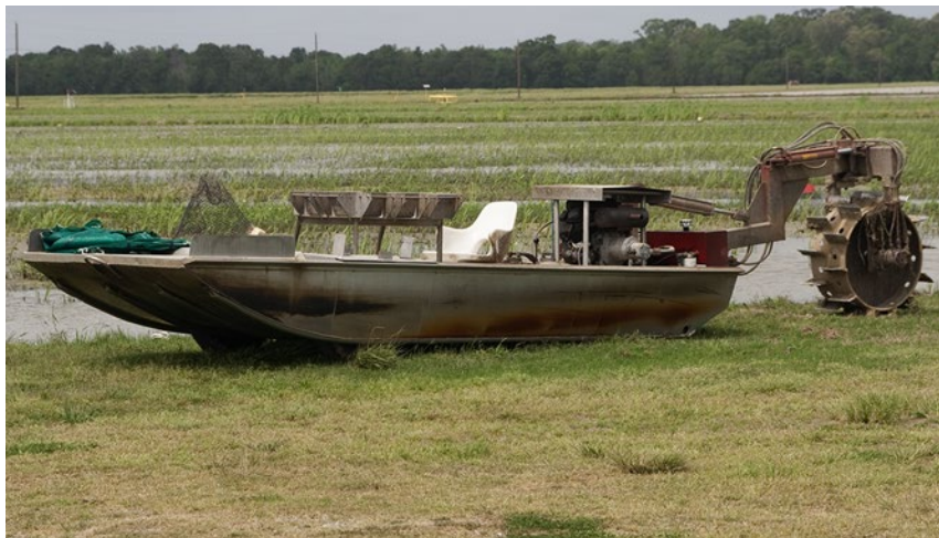
1.4. A crawfish boat parked next to a field. This particular boat was built by Kurt Venable of Rayne. Venable's boats are distinguished by having their forward wheels housed inside the hull of the boat and by the red "Z" shaped steel drive unit which steers the boat at the point of the wheel; other boats either swing the entire drive unit or are hinged at some mid-point.
